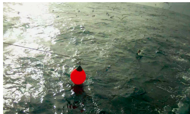
Fig. 4. The 600 mm diameter pinkie, which was previously the only prescribed device to mitigate seabird interactions with trawl vessels, used as the control in trials to test the effectiveness of 2 experimental mitigation devices
