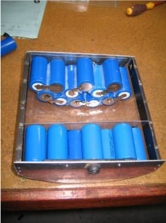
Figure 8. One of the two battery packs for supplying 12 volt power to the cameras and hard drive recorder.
