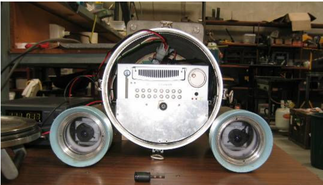
Figure 8. One of the two battery packs for supplying 12 volt power to the cameras and hard drive recorder.
