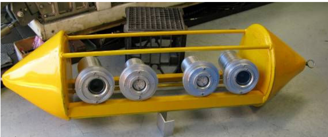
Figure 15. The torpedo shaped stereo-video system used during the fourth round of field trials. The centre two housings hold the light units and the outer two housings hold the video cameras.
