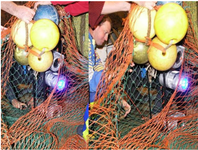
Figure 11. The stereo-video system being sewn into the net.
